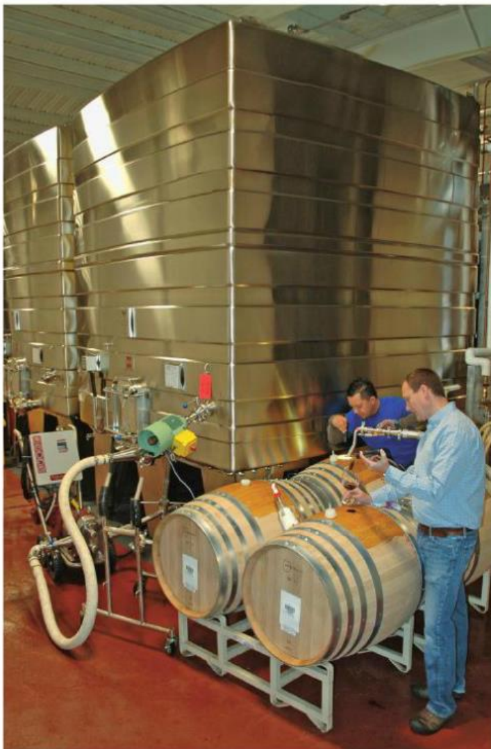
Luis Flores, barrel foreman, racks wine from tank into barrels while Justin Seidenfeld (right) samples barreled wine. Wine from the tank flows through a 3-inch diameter Waukesha variable speed 0 to 130 gpm positive displacement pump with a winged rotor. Four-barrel pallets are used at Rodney Strong Vineyard for best stability in an earthquake.
