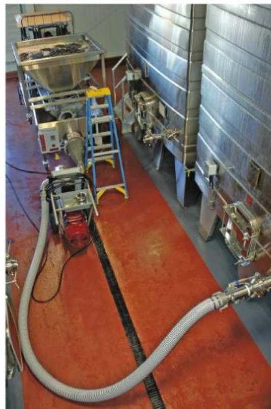
Crush pad with receiving hopper, berry separator/sorter and tank press to use as a basket press.
