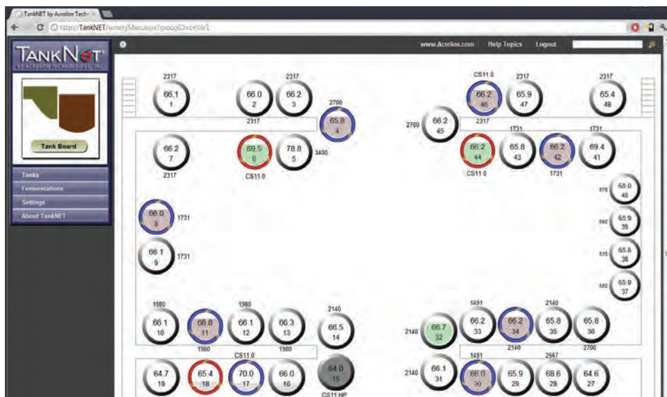
A color-coded system shows each tank's status, which can include fill level, temperature and the last Brix measurement.
