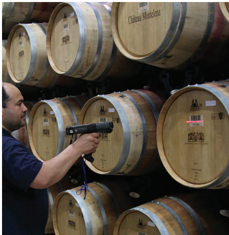
Each barrel at Chateau Montelena is given a barcode sticker. When cellar workers finish a job such as racking or filling, the barrels are scanned and their statuses are updated in the main computer system.
