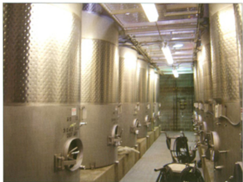
Row of stainless steel barrels used for aging white wines and blending at V. Sattui Winery near St. Helena, Napa Valley.
