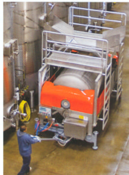
Mobile Diemme press leaves a fermentor after pressing to unload pomace at crush pad.
