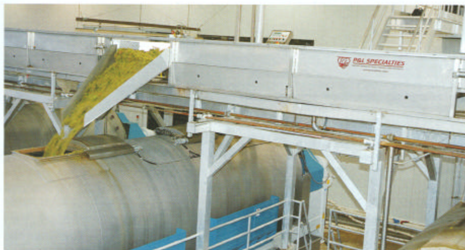
Automated belt delivery system, with variable speed drive, delivers grapes to any press door with a minimum of conveyors and labor required to operate the crush pad.
